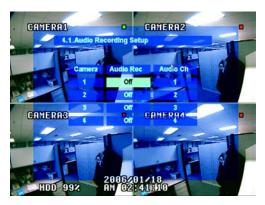
Figure 33. Audio Recording Setup Menu
