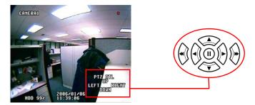
Figure 10. Adjusting PTZ Options on the Monitor
