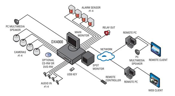
Figure 1. Connecting Devices to the DX4000
