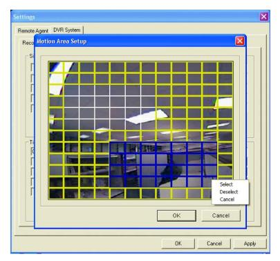
Figure 70. Selecting Partial Regions for Motion Detection
