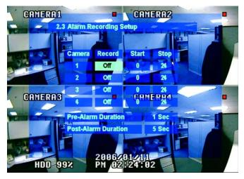
Figure 49. Alarm Recording Setup Menu
