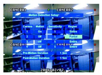
Figure 44. Motion Detection Setup Menu
