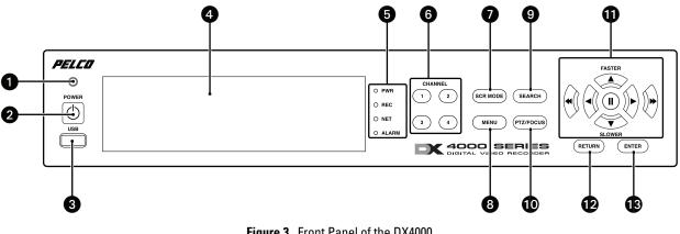
Figure 3. Front Panel of the DX4000
