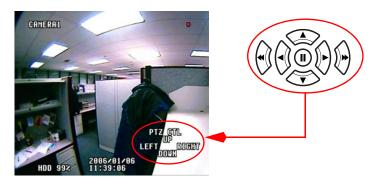
Figure 24. PTZ Control Buttons
