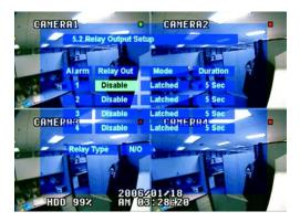
Figure 38. Relay Output Setup Menu
