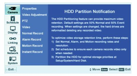
Figure 3. Camera Menu HDD Partition Notification
