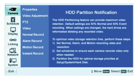
Figure 10. Camera Menu HDD Partition Notification
