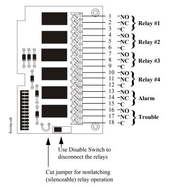
1) Skip a set of dry contacts to maintain the 0.25" required space between powerlimited and nonpower-limited circuits. The wiring of this module must follow the requirements as specified in "Power-limited Wiring Requirements" on page 24.
