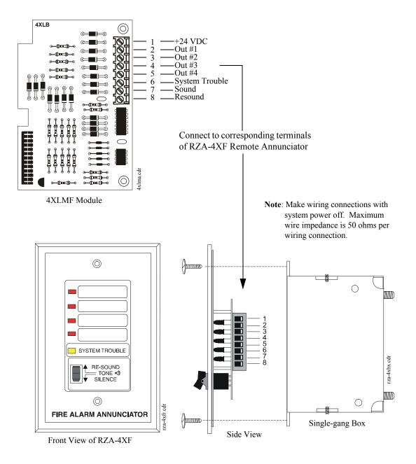
Figure 2.15 4XLMF LED Interface Module
