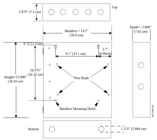
**Figure 2.1 Backbox Mounting Dimensions**
