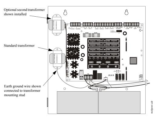
**Figure 2.3 Operating Power Connections**
