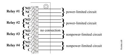
Figure 2.14 4XZMF Zone Relay Module
