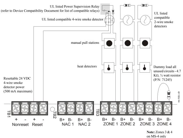
Class B Initiating Device Circuits (supervised and power-limited)  $4.7 \text{ K}\Omega$ ,  $\frac{1}{2}$  watt resistor P/N:71252
