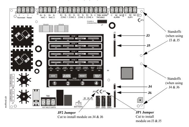
Figure 2.12 4X Option Module Connection to MS-4
