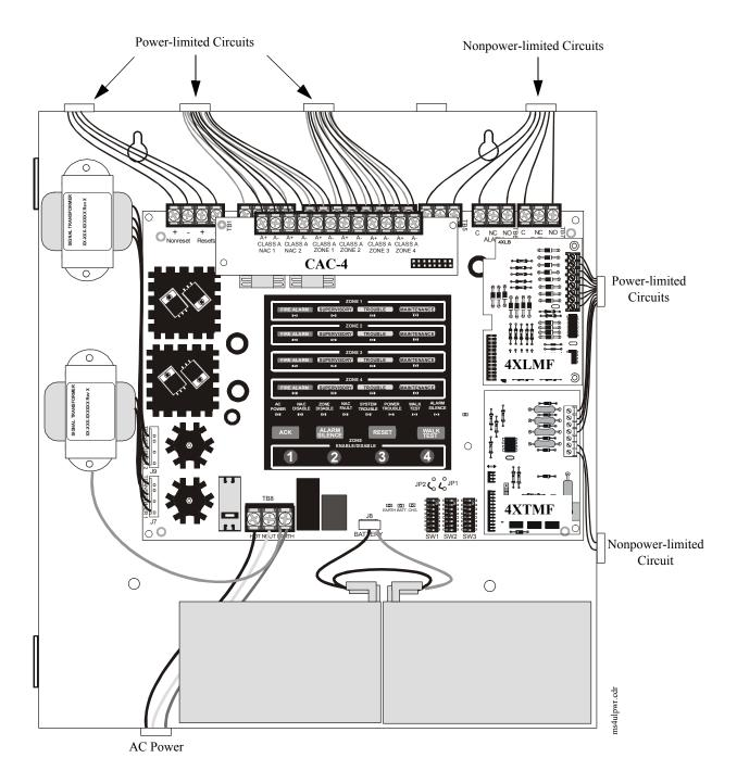
Figure 2.9 Typical UL Power-limited Wiring Requirements
