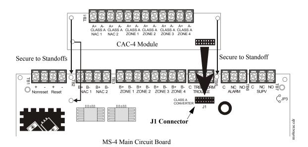
Figure 2.10 CAC-4 Module Installation
