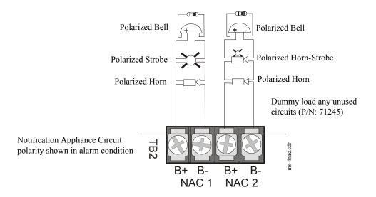
Class B Notification Appliance Circuits (supervised and power-limited)  $4.7 \text{ K}\Omega$ ,  $\frac{1}{2}$  watt resistor P/N:71252
