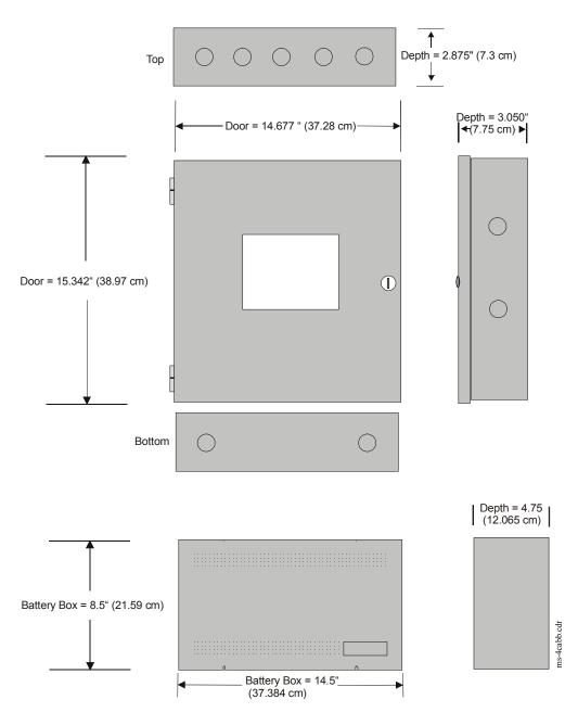
Figure 2.2 Backbox and Battery Box
