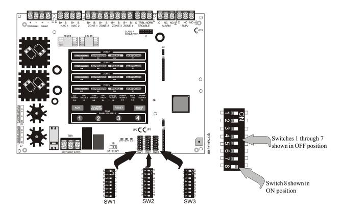
**Figure 3.1 Field Programming DIP Switches**
