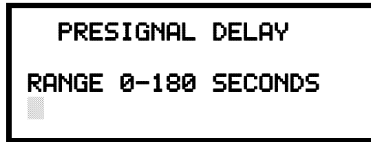
Pre-signal Delay Screen
